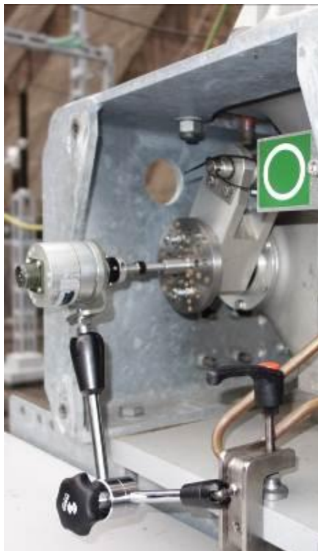
Figure 3. Digital rotary transducer mounted at the 3AP1 FI circuit breaker
